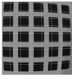
Fig. 4 Test image showing barrel distortion (for the actual camera and lens used).
