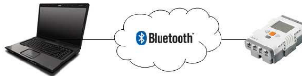
Fig. 4. The client-server architecture used for communication, by means of the Bluetooth wireless protocol, between the computer application (client) and the NXT brick (server).
